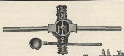
The new Hempy-Cooper Jig pours new main babbitt bearings in the Model "A" Ford cylinder block. Automatically adjustable to the different length bearings. Accurately casts flanges on the rear bearing. No loose bearings, no failures. A two lipped ladle is furnished.
